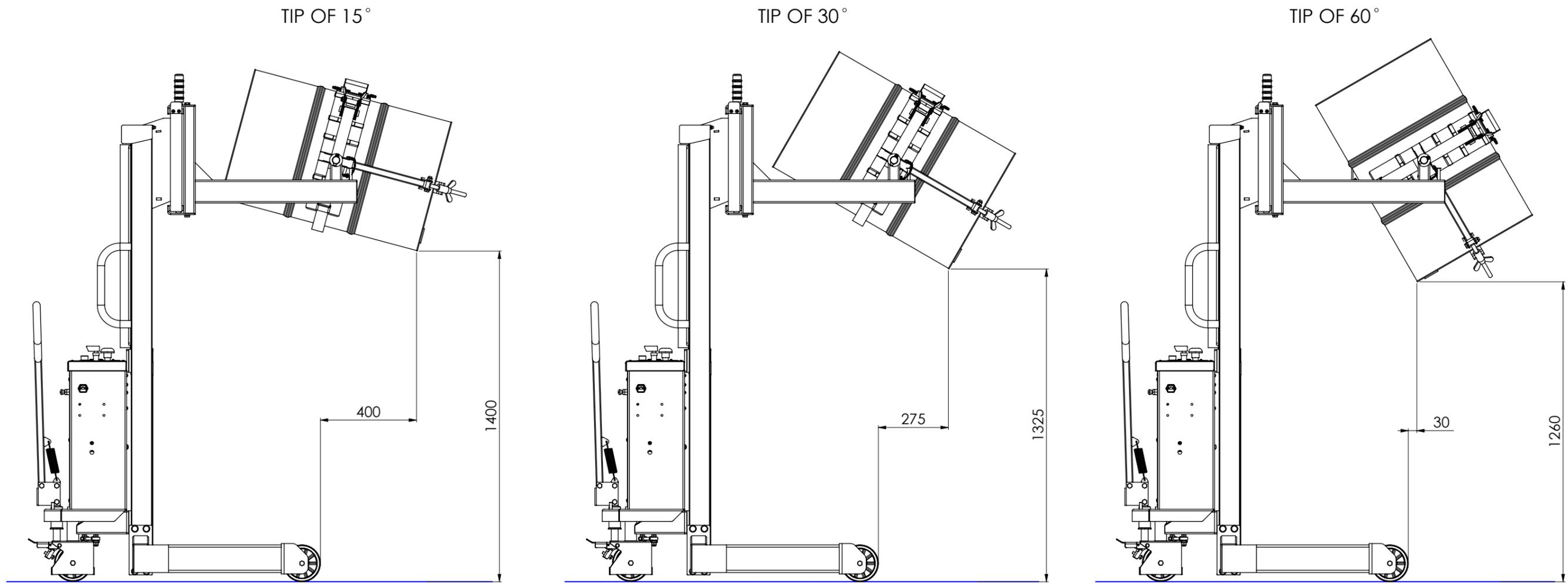
NOTE: STANDARD 205L STEEL DRUM USED FOR TIPPING DIMENSIONS. TIPPING HEIGHT WILL VARY FOR OTHER SIZED DRUMS.
