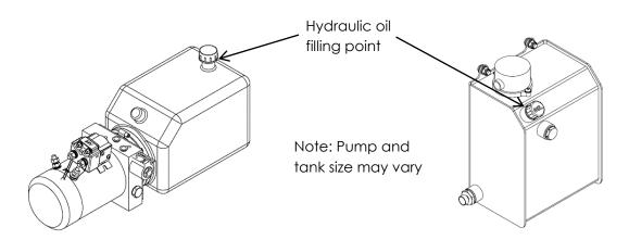
When replacing oil, fill oil to the line or to the middle of the sight glass. Operate all unit functions to their full extents. Return unit head to its lowest position and recheck the oil level, top up if required.
