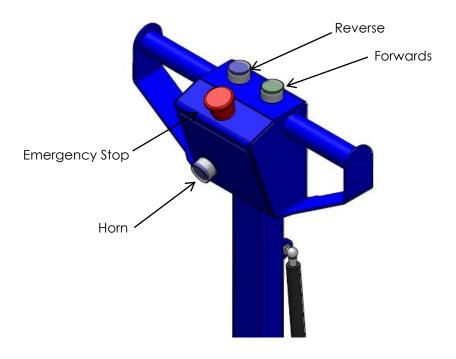
CARE SHOULD BE TAKEN WHEN CHANGING THE DIRECTION OF THE UNIT. WITHOUT LETTING THE UNIT COME TO A STOP FIRST, INSTANTLY CHANGING DIRECTION MAY DAMAGE THE DRIVE SYSTEM.
