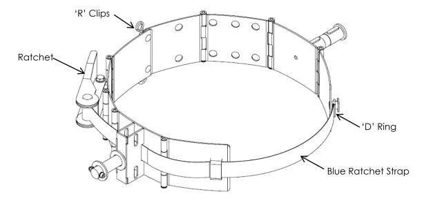
Hook the 'D' ring that is on the end of the blue ratchet strap onto the securing pin,
