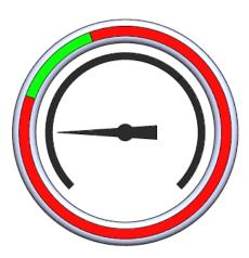
The unit clamps and holds a load in position using friction. The unit is supplied with a pressure gauge to show the clamping force applied to the load being lifted.
