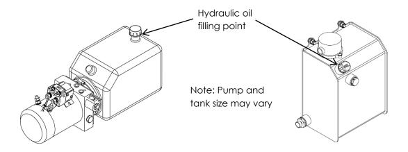
When replacing oil, fill oil to the line or to the middle of the sight glass. Operate all unit functions to their full extents. Return unit head to its lowest position and recheck the oil level, top up if required.
