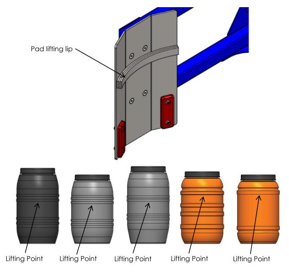
WARNING - DO NOT ATTEMPT TO LIFT ABOVE THE DRUM BANDS OR IN BETWEEN THE DRUM BANDS. DO NOT LIFT A DAMAGED DRUM
