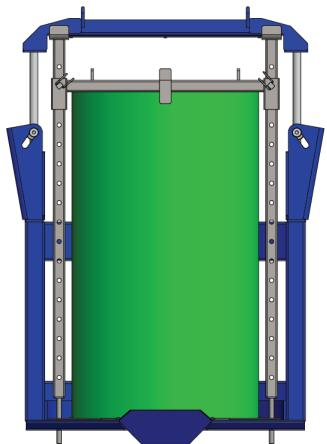
The same procedure as previously mentioned can then be used to clamp the small drum adaptor on top of the drum. Ensure that the drum cannot move around before mixing.
