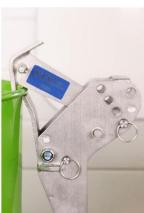
• Ensure the rack is lowered fully so that all the vertical lift stroke is available; this is done by turning the lowering lever anticlockwise.
