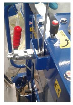
3. Unscrew the clamp bolt by one turn, then test to see if it works correctly. Continue to adjust if required.
