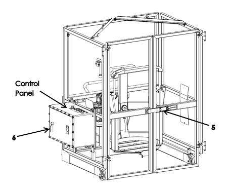
• Close the gate at the front of the unit. Pull the black latching lock with your right hand and slide the stainless-steel bolt (5) across to lock the gates together. Let go of the latching lock to secure the bolt in position.
